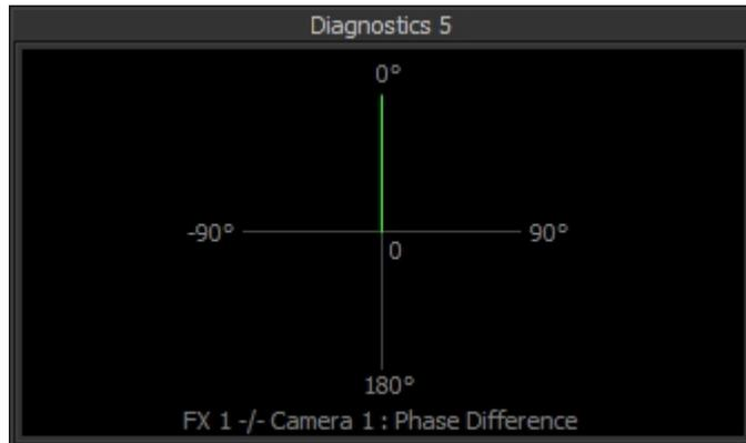
Above image shows a diagnostic with the phase vector steady at 0 degrees, indicating the *FX 1* bus is synchronised to *Camera 1*.
