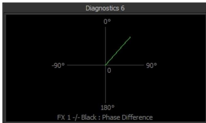
Here the phase vector is slowly rotating clockwise, indicating the *FX 1* bus is not synchronised to the *Black* video signal (internal master clock).
